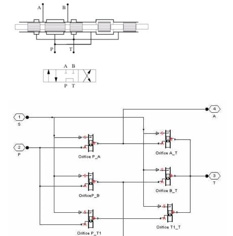
The Orifice with Variable Area Round Holes blocks have been used as a variable orifice in this model. Port T1 corresponds to an intermediate point between ports P and T.
