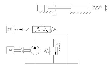
The power unit consists of a motor, a positive-displacement pump, and a pressure relief valve. Depending on its characteristics, such a power unit can be modeled in a variety of ways, as described in "Modeling Power Units" on page 2-26. In this example, the pump unit is assumed to be powerful enough to maintain constant pressure at the valve inlet. Therefore, we are going to represent it in the diagram by an Ideal Hydraulic Pressure Source block.
