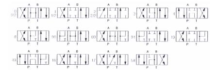
Most of these patterns can be implemented by selecting initial orifice openings in the four-orifice valve configuration shown in the previous section, in the figure named Modeling a 4-Way Directional Valve on page 2-34 (for example, patterns 0, 1, and 3). However, some patterns require a model with six or more variable orifices. For instance, pattern 4 can be implemented with the following configuration, which requires six variable orifice blocks.
