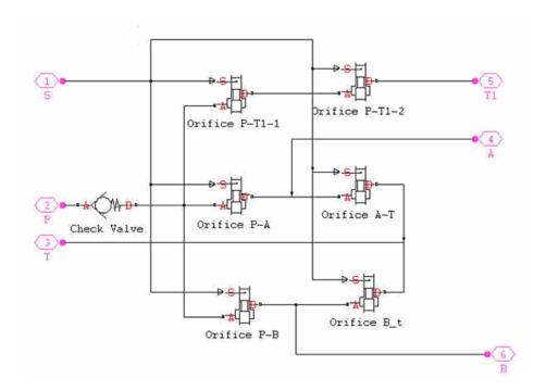
All the orifices in the model are closed (overlapped) in valve neutral position, except orifices P\_T1\_1 and P\_T1\_2. These two orifices should be set open to an extent that allows pump delivery to be discharged at low pressure.
